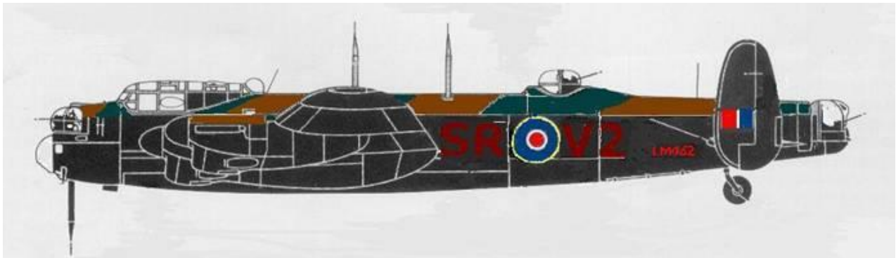
Dessin du SR-V2 muni des 3 antennes ABC. Drawing of the SR-V2 fitted with 3 ABC antennas
